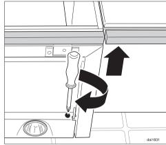
■ The position of the deflector plate can be brought forward by up to 50 mm using the adjusting screws on either side of the deflector plate. Align the deflector plate to the front of the kitchen furniture units on either side.
